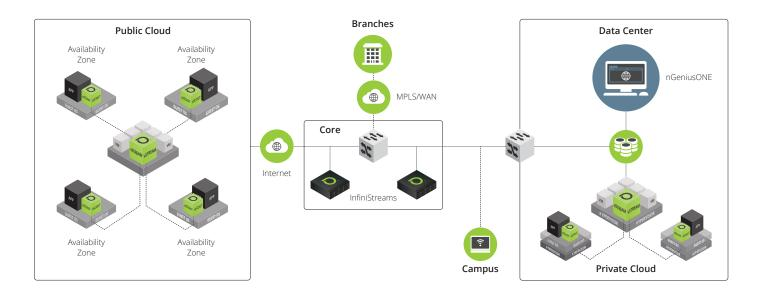
Figure 1: The nGeniusONE platform supports superior analytics from vSCOUT and vSTREAM deployed in hybrid cloud environments. In this case, vSCOUT provides KPIs and forwards traffic on-demand to vSTREAM when deep-dive analysis is required to help identify service health & performance issues.
